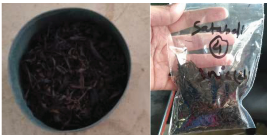
Figure 14. Rice straw biochar prepared under controlled heating and temperature
