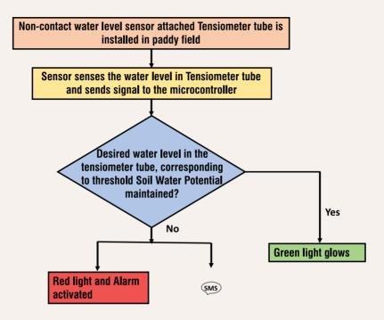
maximising water productivity. As soon as the water level in the tube enters the threshold height the sensor attached to the tube communicates a signal to the microcontroller.
