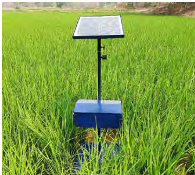
Fig. 1. Eco-friendly Irrigation Alert System (e-IAS) installed in the field
