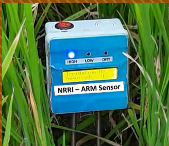
Fig. 2.8. NRRI-ARM sensor installed in the field.
