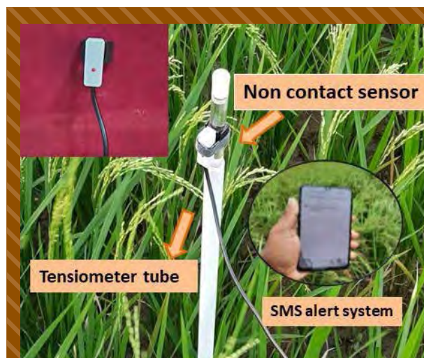
Fig. 2.7. Tensiometer based soil moisture monitoring and irrigation alert system.
