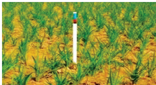
Fig. 18. Color coded tensiometer based irrigation management
