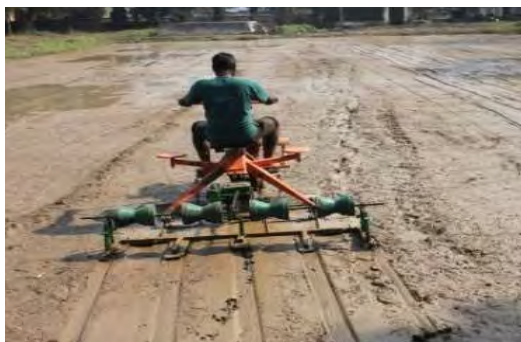
Fig. 14. b. Power drawn drum seeder for sowing sprouted seed in WDSR
