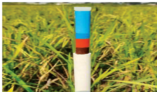
Fig. 19. Color coded tensiometer showing different color bands
