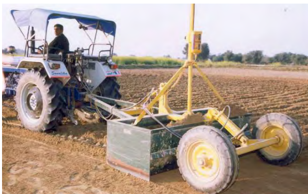
Fig. 3. Laser land leveler in action
