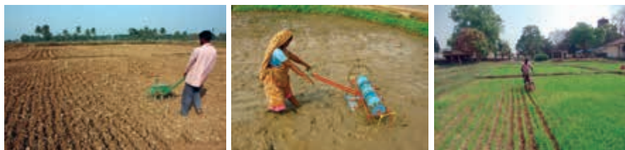
Fig. 9. NRRI developed three row seed drill (a), six row drum seeder (b) and power operated single row dry land weeder (c) in operation.
