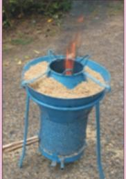
CRRI Chaff and Husk Stove uses 1.2 kg of dry husk and burns continuously for 40 minutes on gasification principle. Cost of the stove is Rs. 550.
