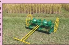
CRRI Six row manual drum seeder (Cylindrical shape) is suitable for sowing of sprouted paddy seed in puddled field at row spacing of 20 cm. Its field capacity is 0.037-0.04 hectare per hour. Its unit cost is Rs. 6500. It reduced seed rate by 35-40% as compared to broadcast seeding and reduced weeding cost about 55%.
