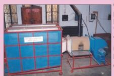
dryer of 125-500 kg capacity. Both raw and parboiled paddy can be dried in this dryer. Drying is accomplished on thin layer principle. The air temperature can be maintained at  $40 \pm 2$ °C throughout the drying period. Paddy at moisture content of 20% was dried to 14% in 6-7 hrs using 10 kg of coal in the furnace. Cost of the
