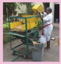
**CRRI Power Rice Winnower cum Cleaner** is a power operated machine to clean threshed paddy crop. Its capacity is 500 kg/hr of clean paddy, having cleaning efficiency of 99%. Cost of the machine is Rs.18,000.
