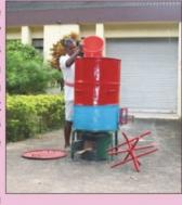
CRRI Mechanical Rice Dryer is a variable capacity batch
