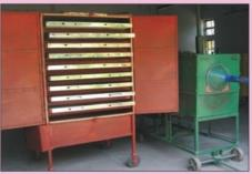
paddy holding capacity. Its main components are drying chamber (LSU type), solid fuel fired furnace with heat exchanger, solar air heaters and blower. Provision is made to connect solar air heaters at the suction end of the blower to supplement with solar heat. One side of the drying chamber is provided with a door for placing trays over the inverted 'V' troughs so that it can also work as a tray dryer for drying
