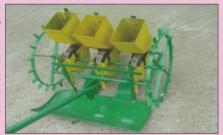
CRRI Four row manual drawn seeder (hyperboloid shape) is suitable for sowing sprouted paddy seed in puddled field at row spacing of 20 cm. Its field capacity is 0.030-0.034 hectare per hour. Sowing with drum seeder reduced seed rate by 60 - 65% as compared to broadcast seeding and reduced weeding cost about 65%. Its unit cost is Rs. 4500.
