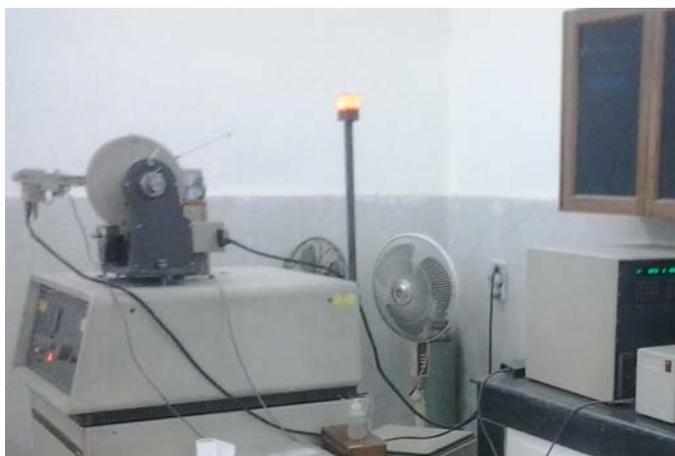
X-ray diffraction set-up used in the experiment
